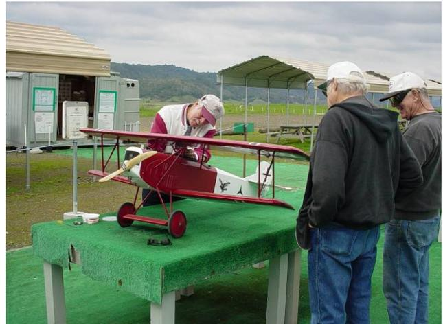
**Larry Miller** built a Fokker DVII model from scale plans and wood cut from a kit cutter outfit a few years ago. The model, with a wingspan of 75", weighing 20 pounds was powered by a ZDZ 40 cc gas engine. It is a beautiful, highly detailed scale model complete with scale pilot, machine gun and an articulated Mercedes Benz engine (1918 Benz that is). The model is so gorgeous that Larry had a problem with it. He didn't want
