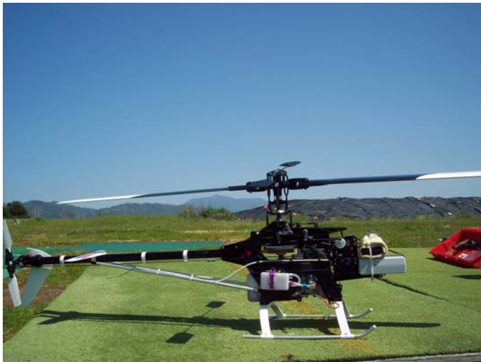
Figure 1. Model Helicopter Raptor 30 Equipped with Telemetry Module.
