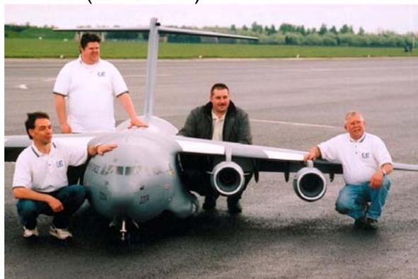
Colin Straus is at the nose of the aircraft. Wingspan is 20 feet 8 inches, and the top of the fin is 74 inches (6 feet 2 inches) above the ground. Takeoff weight is 264 lbs. The rear cargo doors open and they drop an R/C jeep on a pallet, as well as 2 freefall R/C parachutists. The model also has smoke systems on both of the inboard turbines, and uses 2.4 GHz data link to provide real-time data to a laptop computer on the ground while in flight,
