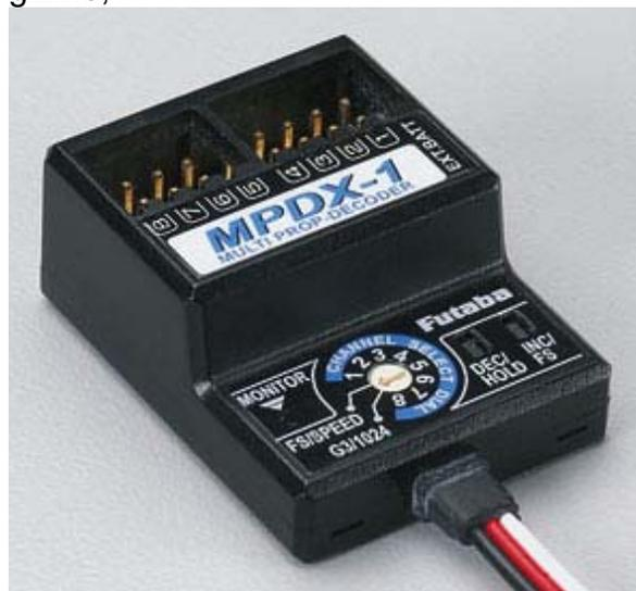
doubles the totals of number of channels to an unbelievable 28! No, this isn't a matchbox which merely lets you connect multiple servos to a single channel, but instead it takes each of the originals binary channels and converts it to 8 proportional, individually accessible channels. Each of the new channels is assignable to a dial or switch. Granted, I couldn't use the 14 I had before, but for a scale guy with lights, guns, doors or whatever, this is way cool!
