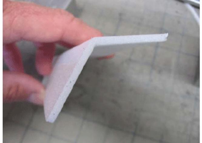
The gap and bevel work together to allow the aileron to hinge at 45 degrees. (A third piece of tape can be used on the bottom for extra support if desired.)
