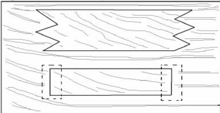
Do not try to simply fill in cracks with glue. Take the time to make tight fitting joints. We are trying to make a sound repair on an aircraft, not calk a submarine. Filling a crack with glue will not hold near as well as a good tight glue joint. The results will be heavy and eventually fail.
