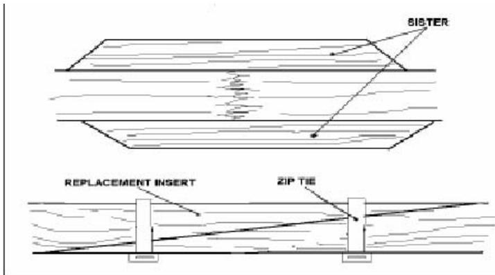
Think of planking the same way as a spar, and avoid butt joints. Cut the patch of planking material with a “zig-zag” at the end of the patch. Then use the patch for the pattern to cut the repair hole through the planking. If there is no room to zig-zag the end of the patch, add a sister under the end of the hole to glue the bottom of the patch to.
