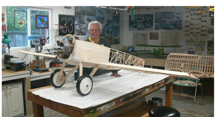
I'm almost finished sheeting the forward fuselage and the top fuselage formers and stringers are done. There are two spruce stringers on each side of the fuselage. The first one has been glued in place. I hope to have the engine mounted in a test stand and start breaking it in shortly.
