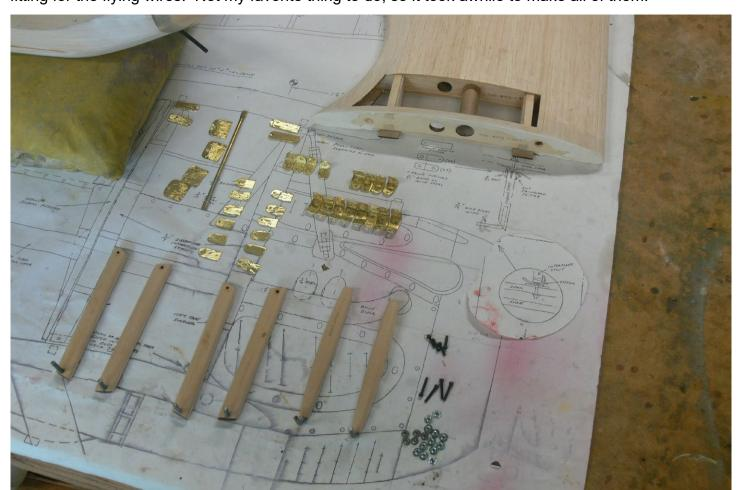
Mounting the fiberglass cowling to the fuselage with eight rare earth magnets and locating dowels to
