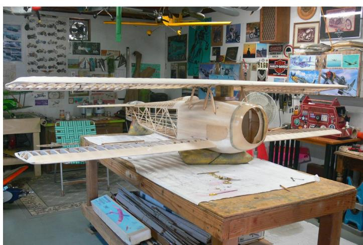
It took over a month, but the Valach twin cylinder 4-stroke engine is broken in. I have just over three hours of run time on it. On the model side I have mounted all the struts and have been working on the control rods for the rudder and elevators. I have a pair of 1/3 scale Vickers machine guns and laid them in the gun troughs just for looks. Next step to fiberglass the forward fuselage and start the covering process.
