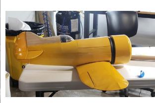
I had issues trying to cut the canopy and it would tend to crack mid-cut. Jake recommended curved scissors to cut and that did it. I didn't have a mm to spare.
